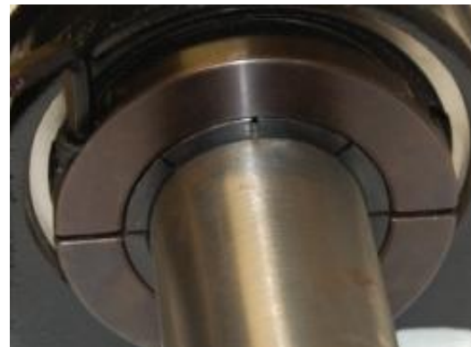
Figure 1) Set screw tightening on a Centrik-Lok bearing
