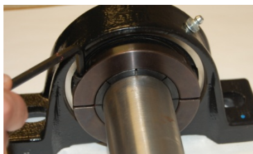
Figure 1) Set screw tightening on a Centrik-Lok bearing
