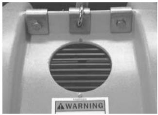
**START UP** — Prior to start up, inspect the Inspection Port installation for proper rotating equipment clearances.
